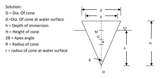
Finding depth of immersion (h) Weight of cone = Weight of water displaced  $\gamma_{cone}V_{cone} = \gamma_{water}V_{water diplaced}$   $0.7x9810x \frac{1}{3}x\pi x R^2 x H = 9810x \frac{1}{3}x\pi x r^2 x h$   $h = \frac{0.7R^2 H}{r^2}$   $h = \frac{0.7(HTan\theta)^2 H}{(hTan\theta)^2}$  h = 0.8879HOG =  $\frac{3}{4}H = 0.75H$ OB =  $\frac{3}{4}h = 0.75x0.8879H = 0.6659H$ BG = OG-OB = 0.75H-0.6659H = 0.0841H
