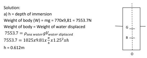
Position of center of buoyancy (OB) = 0.612/2 = 0.306m Position of CG (OG) = 1.8/2 = 0.9m BG = 0.9-0.306 = 0.594m
