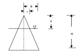
Weight of cone = Weight of water displaced
