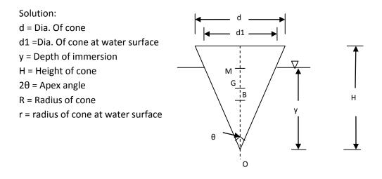
Weight of cone = Weight of water displaced
